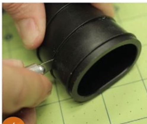
6 The gimbal and battery shelf are attached via 2 shock mounts cut from thick flexible rubber tubing, which helps isolate the camera from propeller vibrations and adds a bit of space, above, to mount the gimbal controller board.
