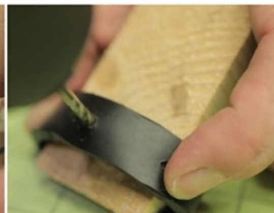
6 The gimbal and battery shelf are attached via 2 shock mounts cut from thick flexible rubber tubing, which helps isolate the camera from propeller vibrations and adds a bit of space, above, to mount the gimbal controller board.
