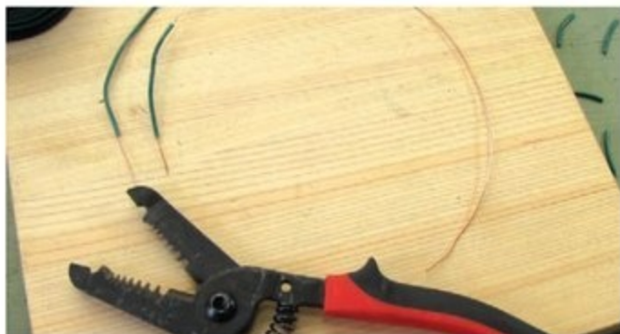
2. Cut and strip the grip and graphite leads.
