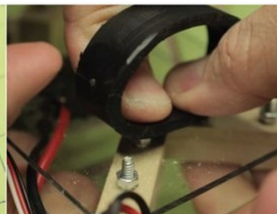
6 The gimbal and battery shelf are attached via 2 shock mounts cut from thick flexible rubber tubing, which helps isolate the camera from propeller vibrations and adds a bit of space, above, to mount the gimbal controller board.
