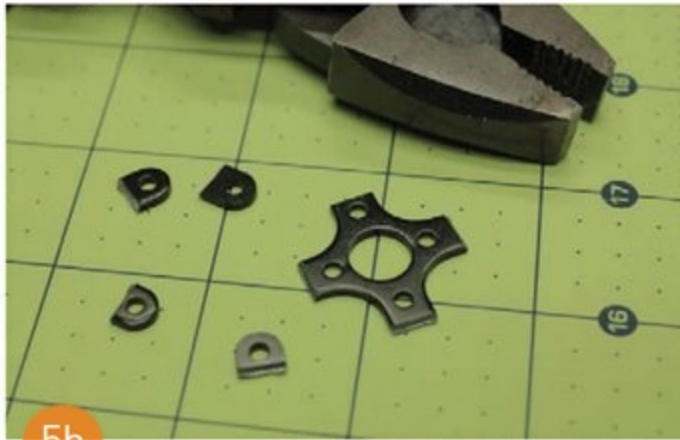
5b Only 2 screws are used on each motor for mounting, and the factory brackets are cut down to save weight.
