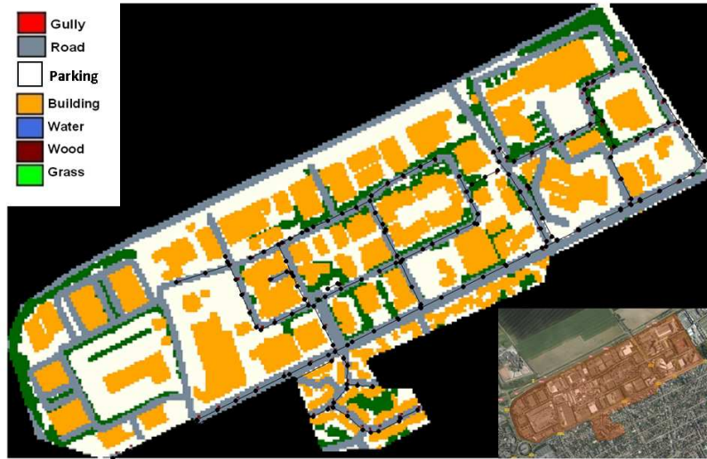
Figure 3: Map of the land use distribution inputted in Multi-Hydro for the Loup catchment with pixels of size 10 m x 10 m. The sewer network modelled with SWMM is superposed to this map (the nodes and conduits are visible along most of the roads). Satellite image the catchment (lower right)
