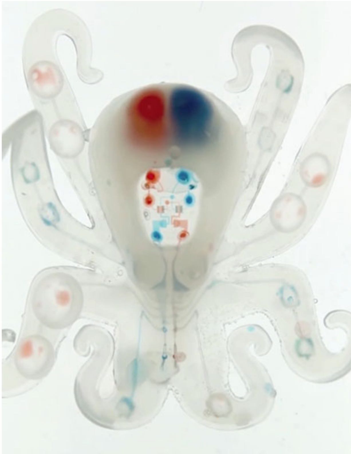
This squishy octopus-shaped machine is one example from the growing field of soft robotics. The Octobot described today is the first self-contained robot made exclusively of soft, flexible parts.
