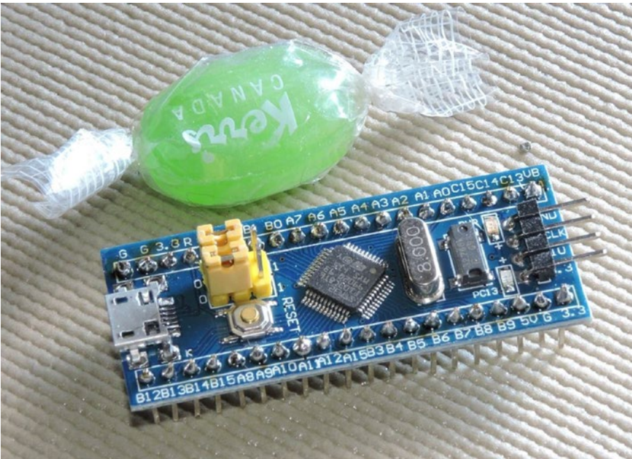
Figure 1-1. The STM32F103C8T6 PCB (printed circuit board) with the header strips soldered in, often referred to as the “blue pill”
