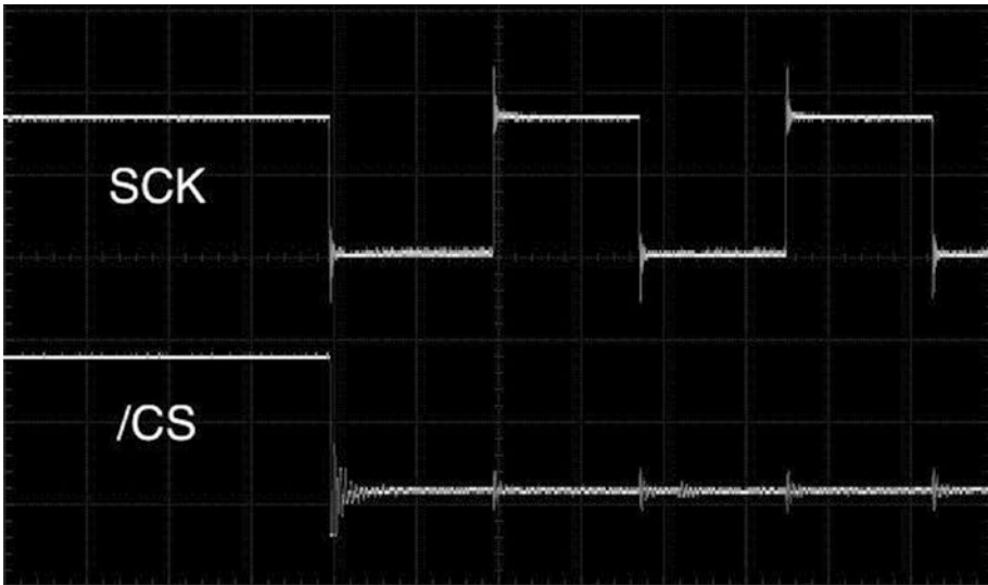
Figure 8-6. DSO trace of SCK and /CS , with SCK idle at low
