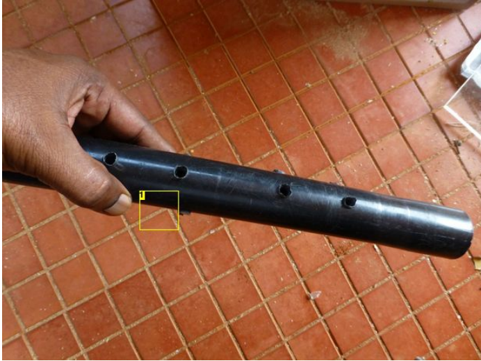
Image Notes 1. Make holes on front and sides
