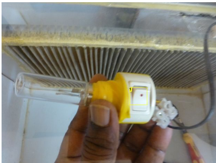
Image Notes 1. Use a holder with a safety switch for UV lamp
