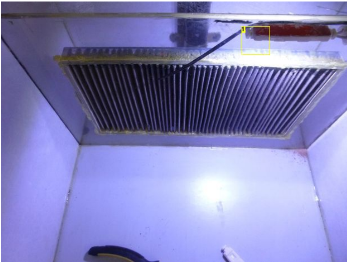
Image Notes 1. fix the LED to the top with Anabond
