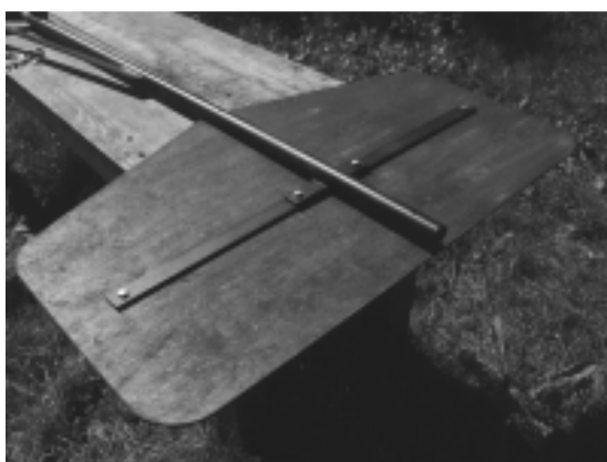
Figure 7 - Tail vane bolted to the tail boom.
