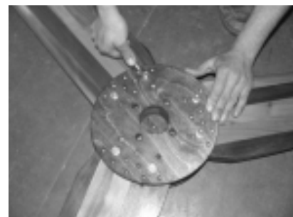
Figure 52 - Re-assembling the rotor for installation.
