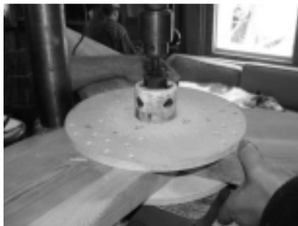
Figure 48 - Cutting the center cavity with a hole saw.
