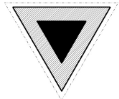
Figure 21 - Footprint of a freestanding tower. The dotted line shows the area that must be cleared of trees and brush, the hatched area is the concrete, and the black area is the tower itself.
