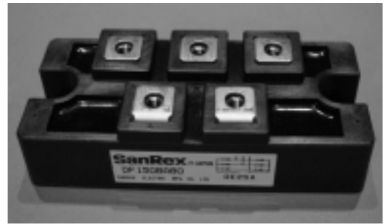
Figure 10 - A pre-made, 3-phase rectifier.
