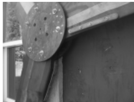
Figure 54 - The two recommended positions for attaching balancing weights to the blades.
