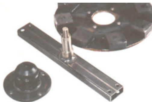
Spine, shaft, hub and magnet rotor
