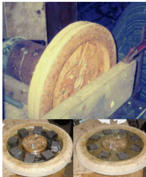
Rotor mould being made and used
