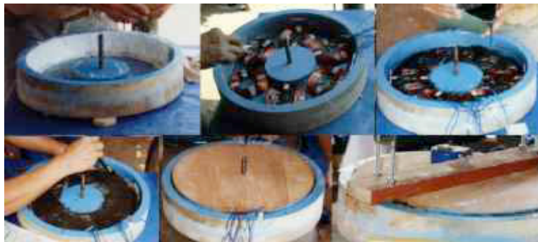
Six stages of the rotor casting procedure
