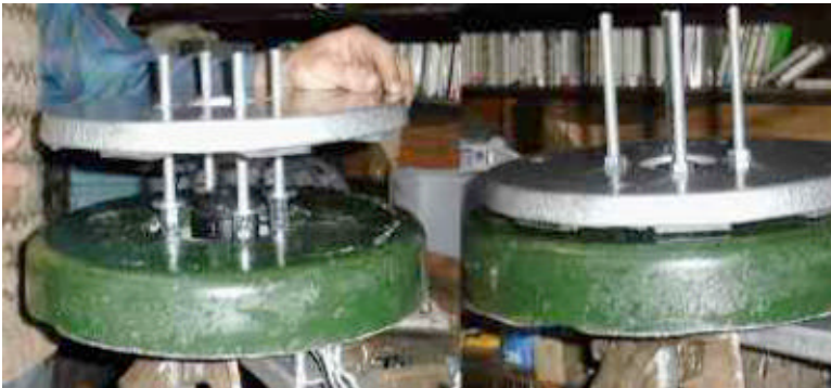
Fitting the front magnet rotor
