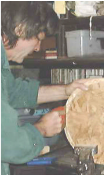
Sawing flat faces on the inner mould
